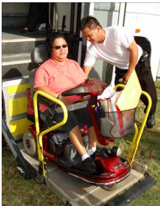
A transit driver practices proper securement techniques on a 3-wheeled power chair as he lowers Evelyn Duenas on the bus power lift.
